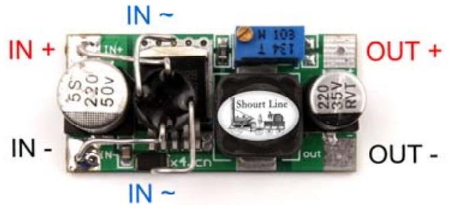
**SL 8453203** Precision Train Throttle & LED controller **\$ 9.95** AC, DC or DCC input + full wave rectifier + 3M mounting pad + 24 in. black input and red/black output cables for motor, loco, car, layout accessories and lighting
