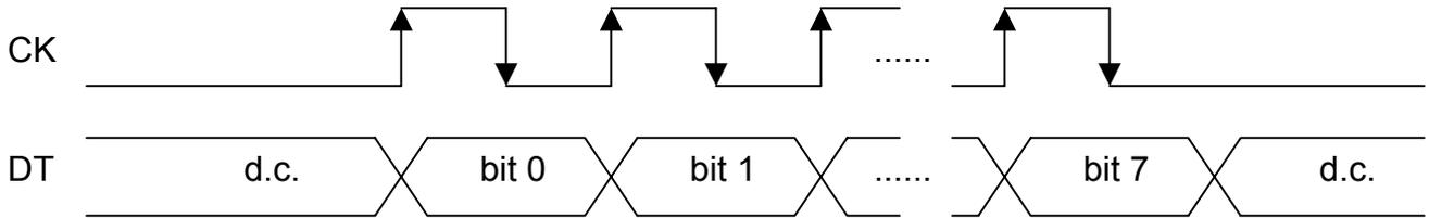
The clock and data lines include a series resistor of 470 ohms at the decoder and on the SUSI-module. The data line must have a pullup resistor to 5 V of  $\geq 15k\Omega$  directly on the decoder's sending device ("before" the 470R). Signal level is 5Volts.
